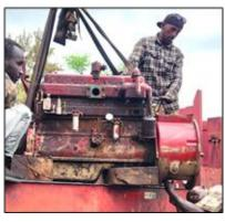
Monte Hininger and the drilling crew spent several weeks repairing the Schramm rig. The picture on the left was taken after everything was completed and the rig was returned to the assigned area to drill. On the right is pictured the rig engine as the clutch replacement assembly on it was being installed. In the picture, on the side of the engine you can
